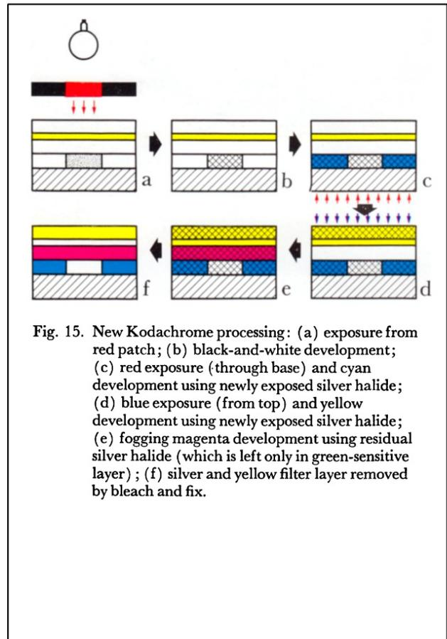
Fig. 15. New Kodachrome processing: (a) exposure from red patch; (b) black-and-white development; (c) red exposure (through base) and cyan development using newly exposed silver halide; (d) blue exposure (from top) and yellow development using newly exposed silver halide; (e) fogging magenta development using residual silver halide (which is left only in green-sensitive layer); (f) silver and yellow filter layer removed by bleach and fix.
