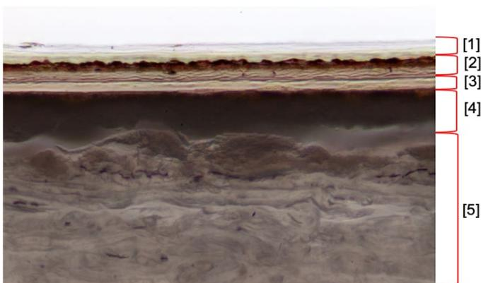
*Figure 10: Cross-section of a Flexichrome in transmitted light. [1] varnish, [2] dyed gelatin relief, [3] gelatin coating, [4] baryta, [5] paper support. Courtesy of the Image Permanence Institute, Rochester Institute of Technology.*
