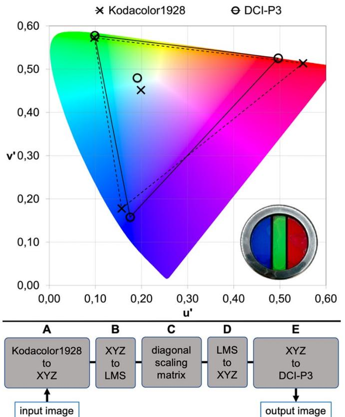
Fig. 6. Top: Chromaticity values of Kodacolor1928 space derived from the transmittances of the filter for projection (reported in the plot) in comparison with DCI-P3. Bottom: The five-step process for the color correction of digitized lenticular films.
