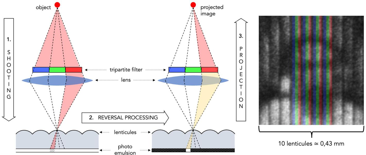
Fig. 2. Kodacolor lenticular film system – Left: Diagram describing the three stages of the lenticular color reproduction—shooting/processing/projection—for an ‘object’ represented by a red dot. Right: Front view of the processed photo-emulsion with superimposed stripes that indicate the location of the color separations.
