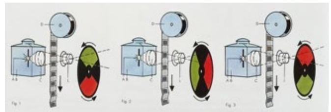
*Fig. 6 – Vitacolor used the same principle as the earlier Kinemacolor process, illustrated here (Coote, 1993)*
