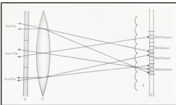
*Fig. 5 – Diagram illustrating the lenticular process (Coe, 1981)*
