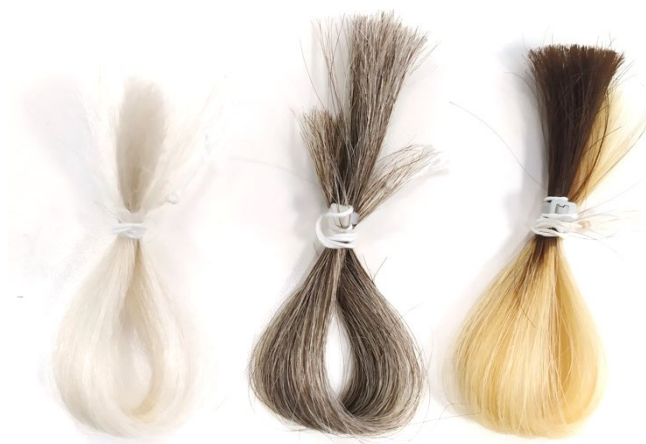
Fig. 1. Samples of the different swatches: yak hair ( S_1 left); 80/20 mixture ( S_2 middle); bleached 4.0 ( S_3 right - original 4.0 can be seen at the top).
