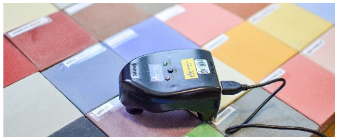
Fig. 1. Use of the colorimeter on the tiles from Paço and the sample from the Fábrica de Mosaicos.
