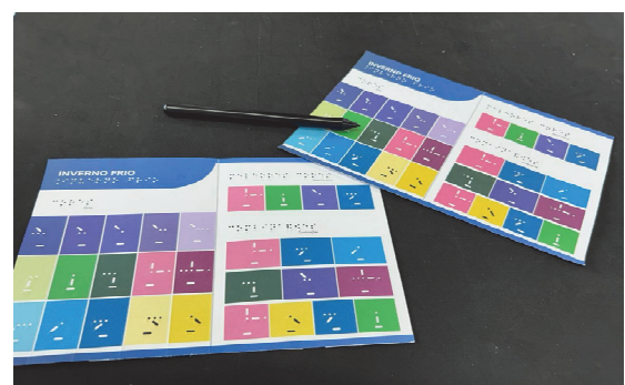
Fig. 6. Printed prototype of the tactile color chart.
