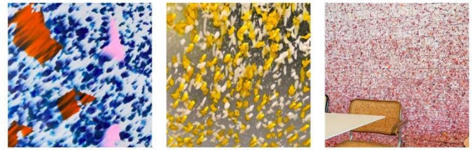
Fig. 4. Finishings. From left to right: Polygood by The Good Plastic Company (Netherlands), Plastiz (Italy), Fab_Brick (France). The first two images show the results of the thermo-pressing process, made by using the “sheetpress” machine. The bricks made by Fab_Brick in the third image are still representing an output of a process that uses pressure but combined with glue rather than high temperatures. The general output given by pressing process of the three projects is related to the “confetti” aesthetics.
