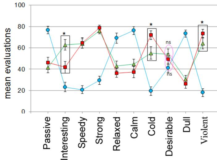
Fig. 4. Mean evaluations given by the participants to the semantic scales as a function of the three light sources. Blue circles: halogen lamp; green triangles: LED-A; red squares: LED-B.
