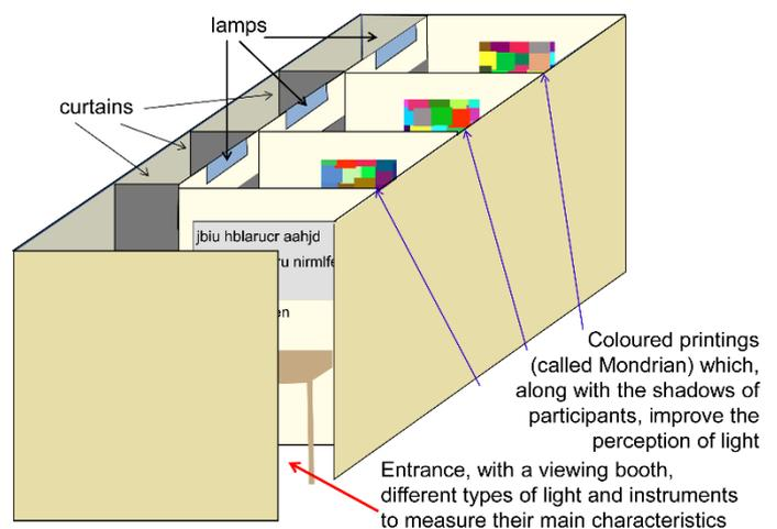
Fig. 1. The rooms where the experiment has been performed.
