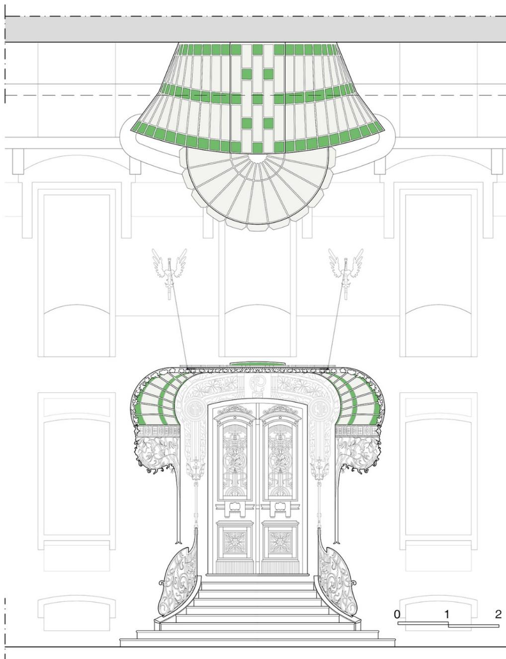
Fig. 5. Plan and elevation of the entrance portal with the wrought iron canopy with two-coloured glass, original scale 1:50.
