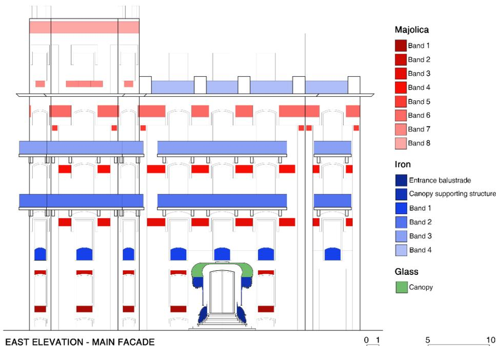
Fig. 4. Distribution scheme of the facade of Villa Pappone with indication and position of the decorative elements declined according to the material.
