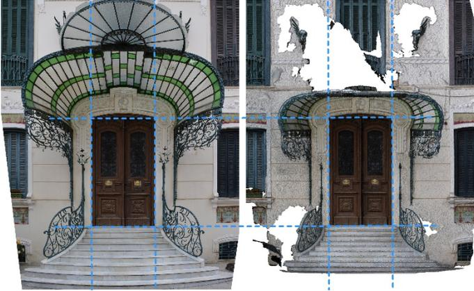
Fig. 6. Comparison between a perspective view from a photograph of the canopy and the orthogonal view of the textured model obtained with photogrammetry.
