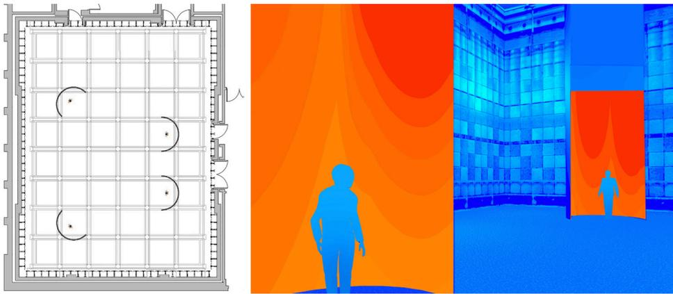
Figure 1 - Semi-circular viewing chambers (tubicles), size: 2.75 m diameter x 4.25 m height, in a 15.25 m x 18.30 m x 10.56 m black box studio space
