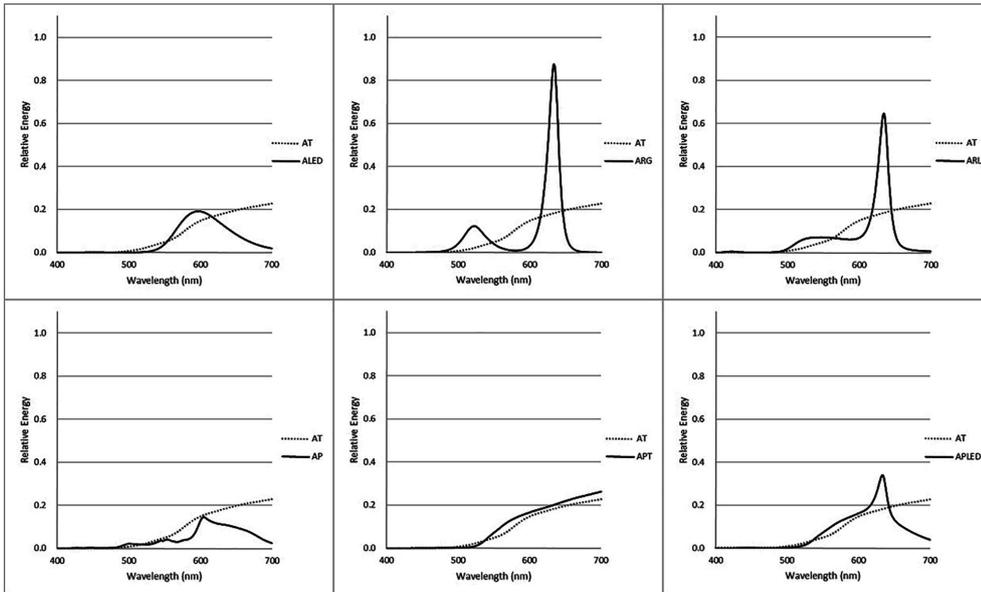
Figure 2 - Spectral power distributions of amber conditions 2-7 in relation to condition 1 (scaled for relative light level).
