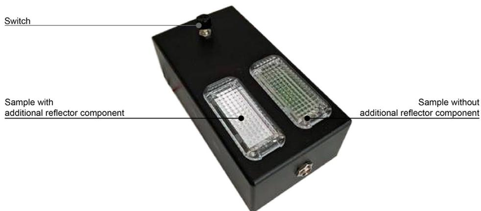
Figure 4 - Demonstration device for optical measurements and validation
