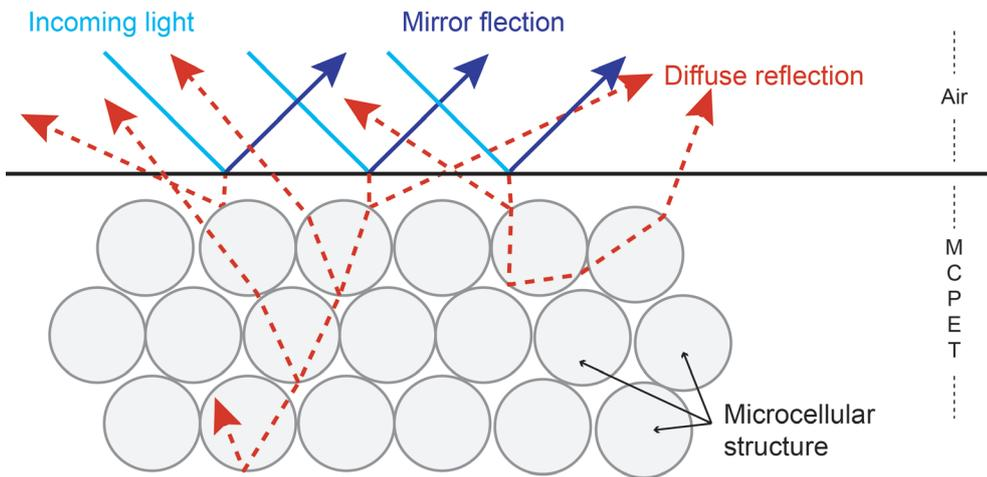
Figure 2 - Internal structure and reflective behaviour of MCPET
