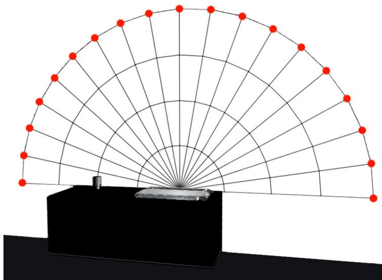
Figure 5 - Illuminance measurement with the demonstration device
