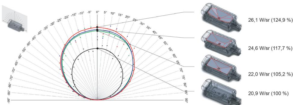
Figure 3 - Results of an optical simulation. The black curve is the result of the original assembly, the other three curves show the results where the samples contained a new reflector geometry
