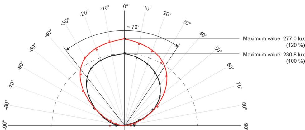
Figure 6 - Measurement results of the two lamps (black: original sample, red: sample with the additional component). Along about 70° range the optimized lamp has greater result than the maximum value of the original one which is presented with the dashed curve.
