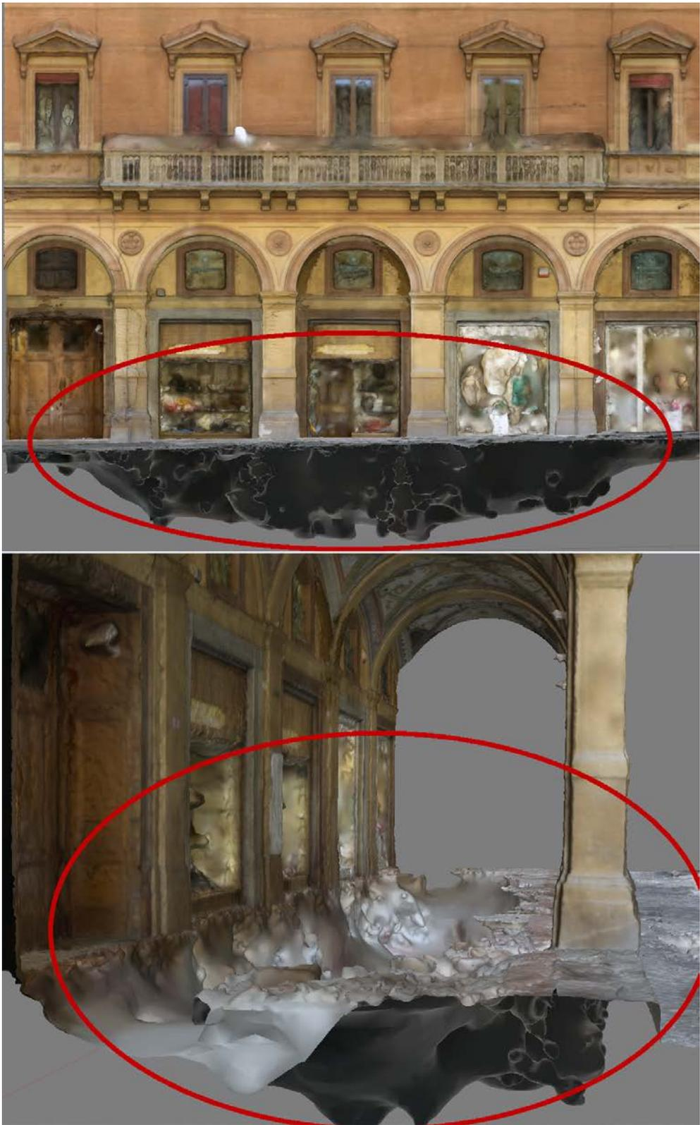
Figure 1 - Typical problems of the automatic photogrammetry pipeline in presence of specular effects
