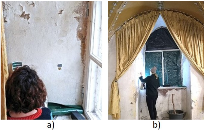
Fig. 5. The participants determining the colours of the paint patches in a) daylight and b) under a spotlight.
