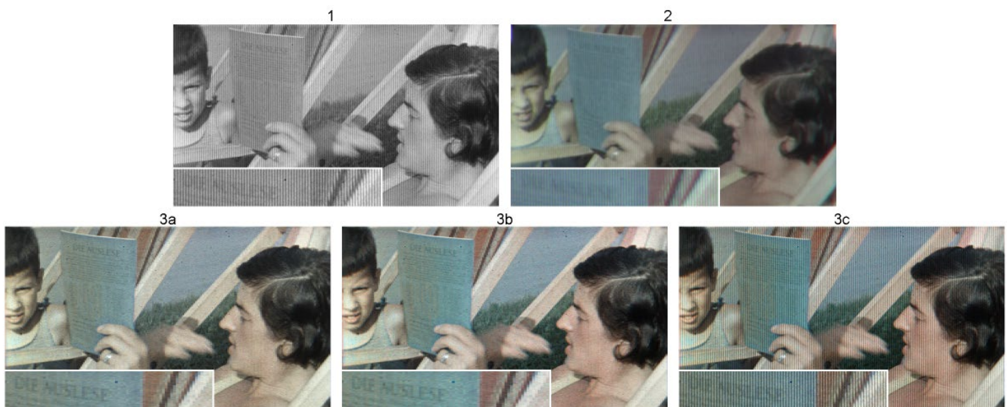
Fig. 7. Digital images of a lenticular film frame with inset enlargement. 1 : Black-and-white scan of the film emulsion. 2 : Slit scan. 3a : Output of deep-doLCE. 3b : Output of deep-doLCE after color correction. 3c : Merge of luminance from 1 and chrominance from 3b.
