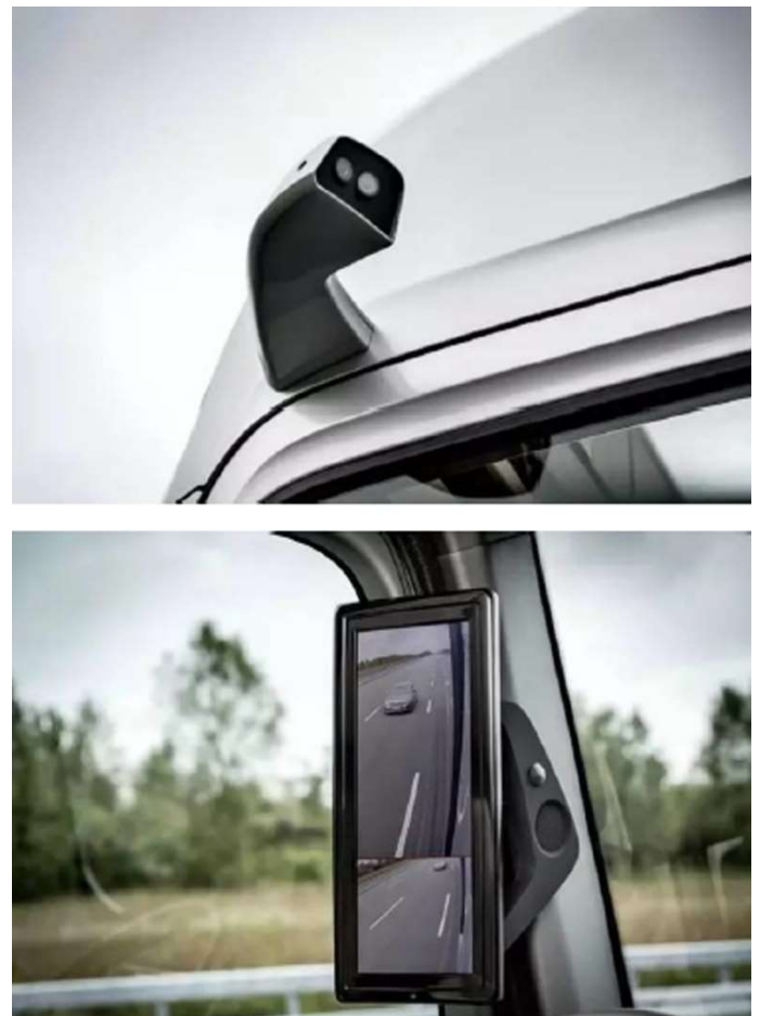
Fig. 1. Example of a CMS system for a truck. Top row: CMS camera, bottom row: CMS display
