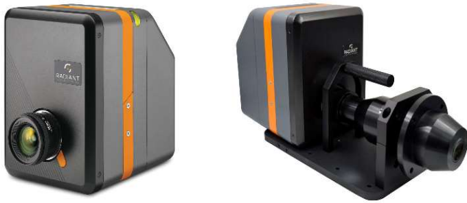
Fig. 3. Example of a 2D colorimeter, used for CMS evaluation. On the right, the colorimeter with a conoscopic lens mounted.
