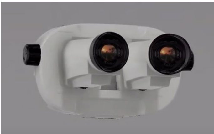
Fig. 1. The MR system compatible stereoscopic visor has two OLED displays and integrated eye-tracking cameras to both real-time visual monitor and record direction of gaze and pupil diameter.
