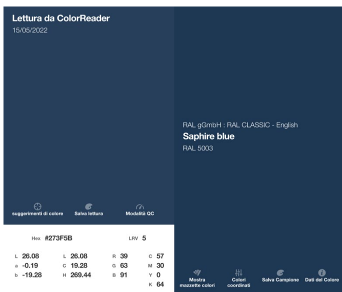
Fig. 2. Screenshot of a DataReader color measurement. The corresponding RAL code is provided by the ColorReader application as the closest RAL color sample.
