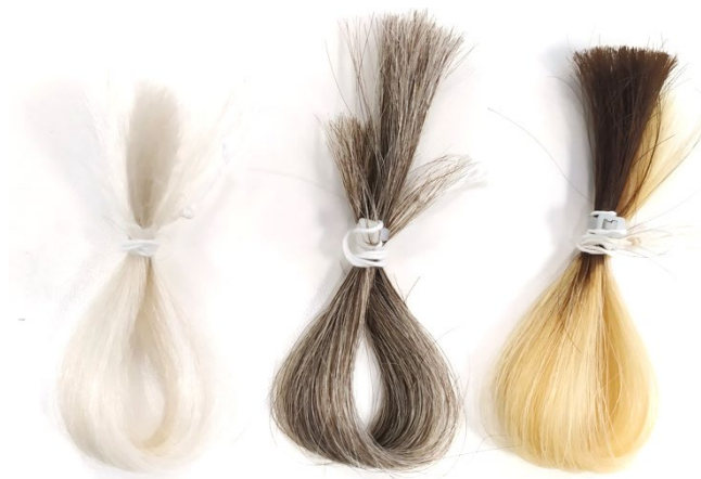
Fig. 1. Samples of the different swatches: yak hair ( S_1 left); 80/20 mixture ( S_2 middle); bleached 4.0 ( S_3 right - original 4.0 can be seen at the top).
