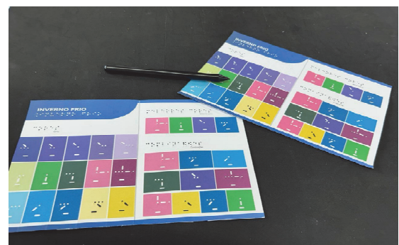
Fig. 6. Printed prototype of the tactile color chart.
