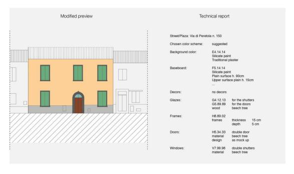
Fig. 4. Facade unit diagram and related technical report.
