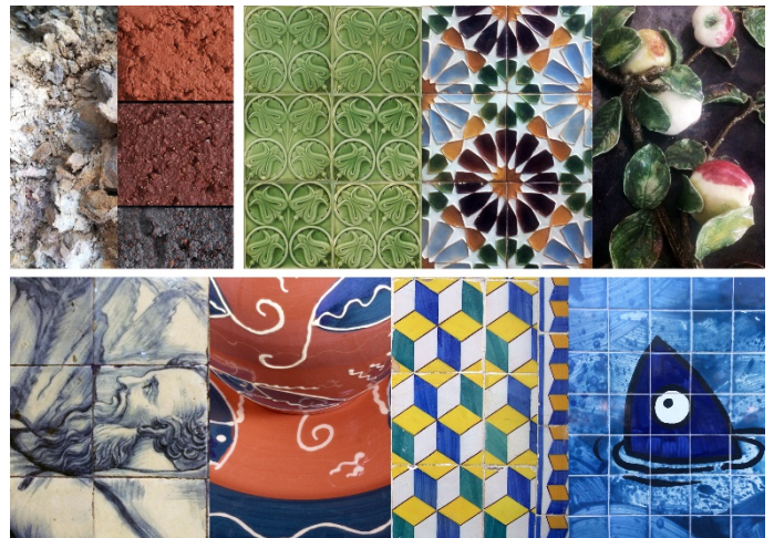
Fig. 1. Ceramic colour features (top, from left to right): a. Ceramic raw materials and the effects of temperature on the ceramics' colour body; b. ornamental patterns with glazes (transparent, semi-transparent and opaque glazes). Other decor techniques (bottom, from left to right): hand painted in-glaze pigment; slip pipette underglaze; stencil brush; brush on fired glaze. Photo: Carla Lobo.
