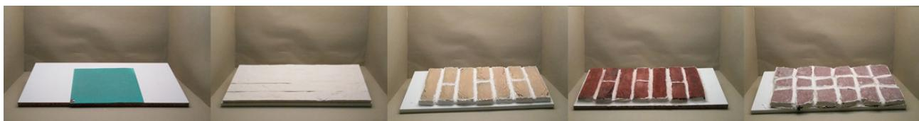
Figure 2 - Selected urban materials for the experiment from left to right: Oxidated Copper Green, Ostuni Natural Stone, Brick Forum Oro, Brick Fermette Cod 160, Porphyry Stone
