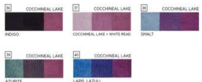
Fig. 6. Purple samples. 36) Cocchineal lake over indigo; 37) cochineal lake over a mixture of such lake with white lead; 38) cochineal lake over smalt; 39) cochineal lake over azurite; 40) cochineal lake over lapis lazuli
